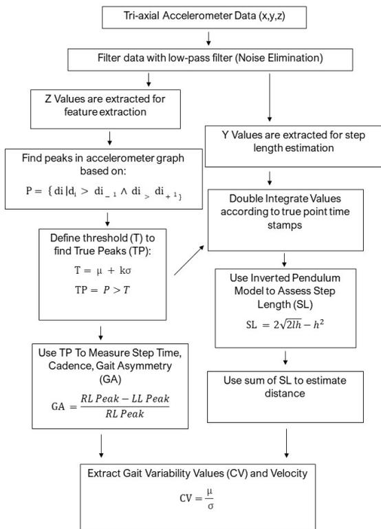
Figure 5: Representation of algorithm in flowchart form
